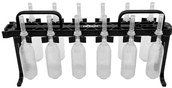
Figure 6 - Cartridge Rack with Cartridges nRicher Cartridges shown in the Cartridge Rack; the Capture Tube is removed and placed in a separate rack when accessing the Sample Tube portion of the nRicher Cartridge.
